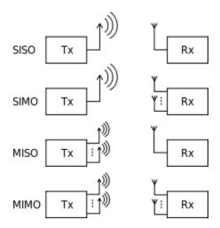
Understanding of SISO, SIMO, MISO and MIMO. Using multiple antennas and transmitting in different frequency channels can reduce fading, and can greatly increase the system capacity.
